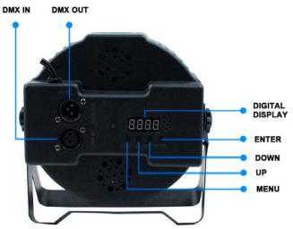
Operation instructions: Press function Button MENU will cycle out nine different function effects, the first two digits of the digital tube represent the current function (refer to the function table). The last two digits represent the parameters of the address code or speed at which the function is located. Press UP or DOWN to modify its parameter value. Then press ENTER to confirm.
